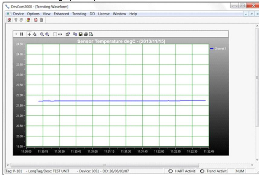
The user can manipulate the graph as desired. “Tracking” is the term used to describe how the graph control follows the data, changing the axis in real time so that all of the data is shown. Below are the specific parts of the graph:
