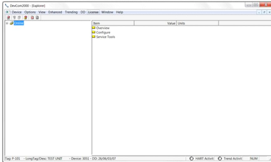
The left pane of the window shows the menu structure and the right pane of the window displays corresponding parameters of the menu selected. The DevCom2000 screens shown in this document are only an example of what you may see when connected to your field device. What you see is actually controlled by the devices DD file and the device. Hence, the menus, data, status and configurations displayed are specified by the field device's manufacturer when they release the devices DD file.
