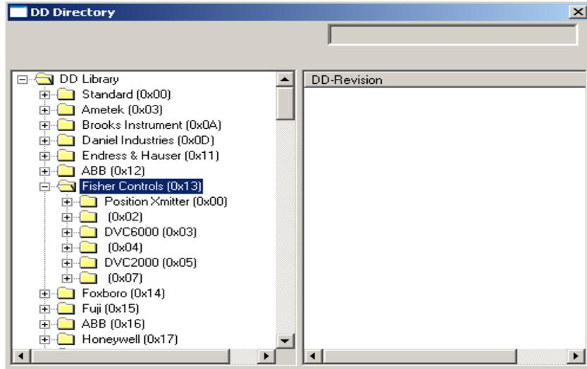
The manufacturer ID of Fisher Controls is 000013. Device IDs 0002, 0004, and 0007 all do not have a label. This is when updating a DD label is useful. To update the label perform the following steps:
