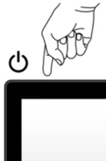
If the tablet was previously shut down it will boot up Windows. If the tablet was previously asleep it will immediately reawaken. If the Tablet does not respond the battery may be too low.
