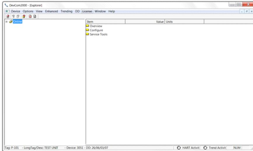
The organization of the data in this explorer-style window is dictated by the device DD. The left hand tree-pane of this window shows the logical groups of field device data. These are called "Menus". The right hand data-pane shows the data, any sub-groups and any standard operating procedures found on a given menu.
